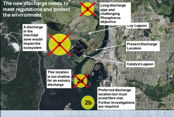
1 Long discharge pipe and challenging Phosphorus objective
