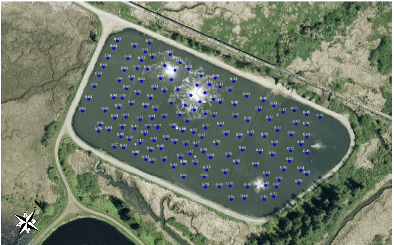
Photo 2. An overhead view of the Sewage Lagoon. The points (blue) represent each profile location and associated sludge depth at that point. The aerators are not represented as they are mobile throughout the lagoon along cables.
