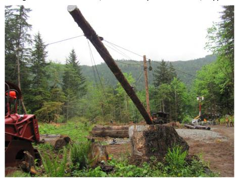
Photo 3. The spar tree was moved, re-rigged and stood up at its new location by JJ Logging and crew (Photo by David Hooper).
