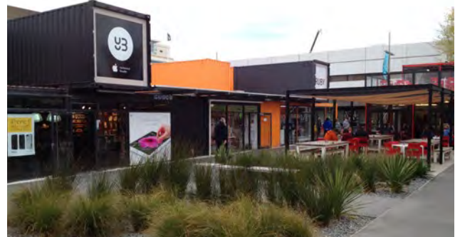
Christchurch Re:Start Mall was established from shipping containers after the earthquake as fast way to provide economical space for businesses.
