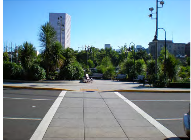
Changes in paving texture and colour can help signal to both pedestrians and motorists that there is a change in travel patterns.
